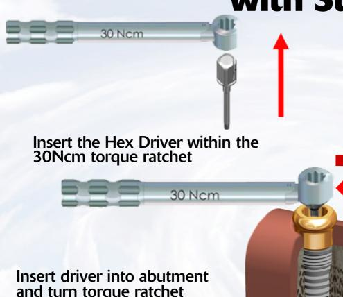
Insert driver into abutment and turn torque ratchet clockwise until torque of 30 Ncm is reached and the head of the ratchet releases
